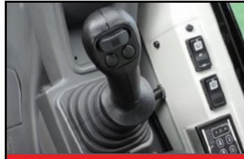
Pilot Operated Controls
