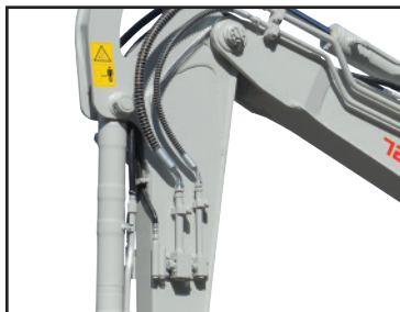
Auxiliary Hydraulic Lines
