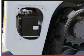
Battery Access Panel
